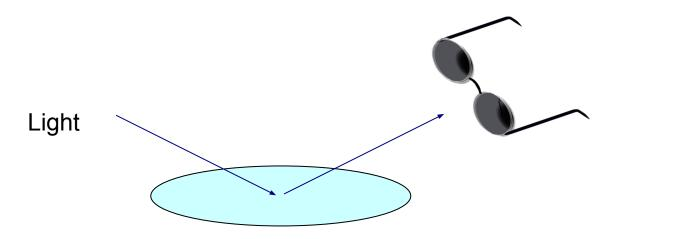
Sunlight has equal amounts of vertical and horizontally polarized light. But more of the horizontal component is reflected by the surface. Polarized sunglasses can block that component selectively, reducing glare!
