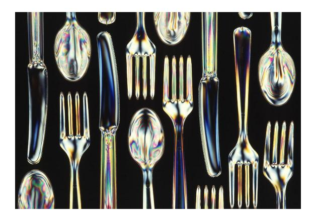
Polarized light can be used to visualize plastic materials under stress, and predict where they will fail.
