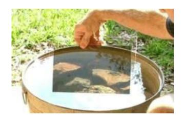
Sunlight has equal amounts of vertical and horizontally polarized light. But more of the horizontal component is reflected by the surface. Polarized sunglasses can block that component selectively, reducing glare!
